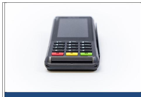
The EMV slot is located on bottom of the device. Please inspect it to make sure that no foreign devices are attached or inserted, and ensure that the area is free of any obvious tamper marks such as tool marks.
