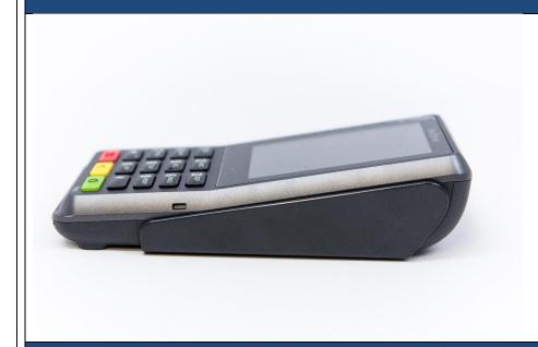
The right side of the device the MSR slot. Please inspect it to make sure that no foreign devices are attached or inserted, and ensure that the area is free of any obvious tamper marks such as tool marks
