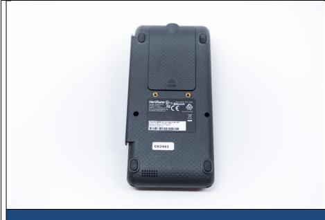
The back of the device contains the device model and serial number as well as a removable compartment for the units power/data cable and MicroSD memory optional components.
